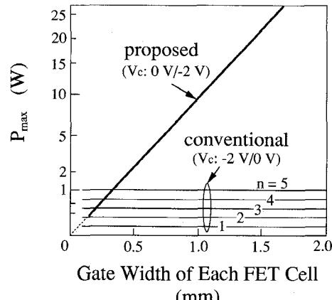
Fig. 3. Maximum transmit power comparison between the proposed LC-resonant T/R switch and conventional series/shunt FET T/R switches in 2-V operation, where  $I_{\text{dss}} = 0.2 \text{ A/mm}$ ,  $V_p = -1 \text{ V}$ , and  $Q_L = 0.44$ .
