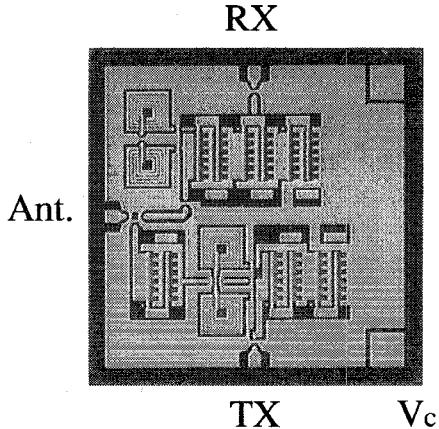
Fig. 6. Photograph of a fabricated LC-resonant T/R-switch MMIC.
