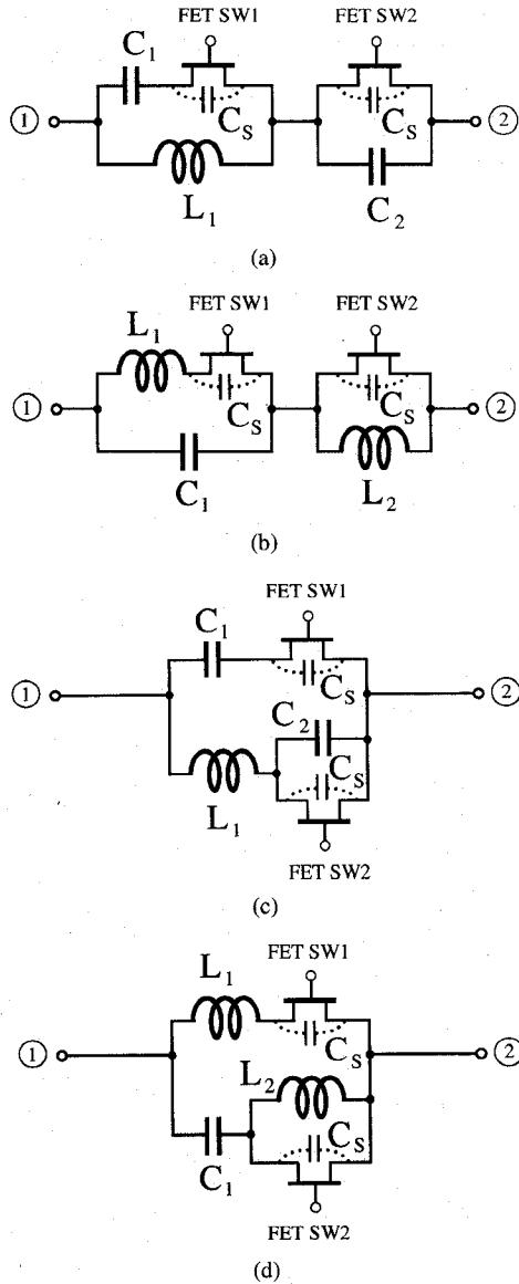
Fig. 4. FET-switchable LC-resonant circuit schemes.
