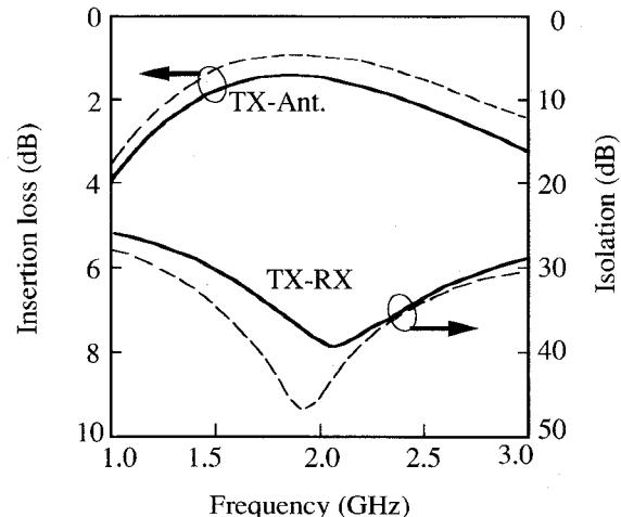
Fig. 8. Frequency response of the LC-resonant T/R switch in the transmit mode (solid lines: measured; dashed lines: calculated).  $V_c$  is 0 V.
