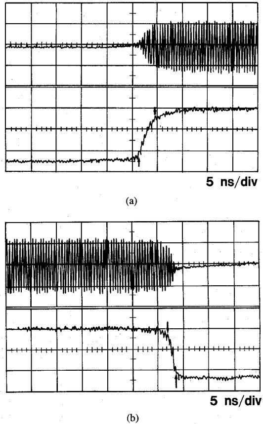
Fig. 12. (a) Rise and (b) fall time characteristics of the LC-resonant T/R switch.
